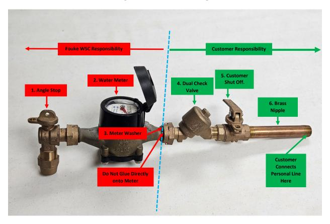
The blue dotted line shows the division between the Corporation's ownership and the customer's ownership. A dual check valve, ball valve and brass nipple are installed upon new installation. It is required for all customers to maintain and replace when necessary.
